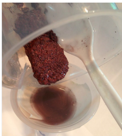
Figure 2. Transferring the copper into the filter funnel
