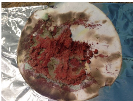
Figure 5. Dry Copper metal powder from oven-dry method
