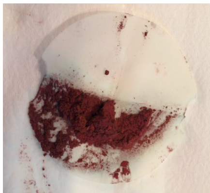
Figure 4. Unfold the filter paper and lay it flat on paper towels
